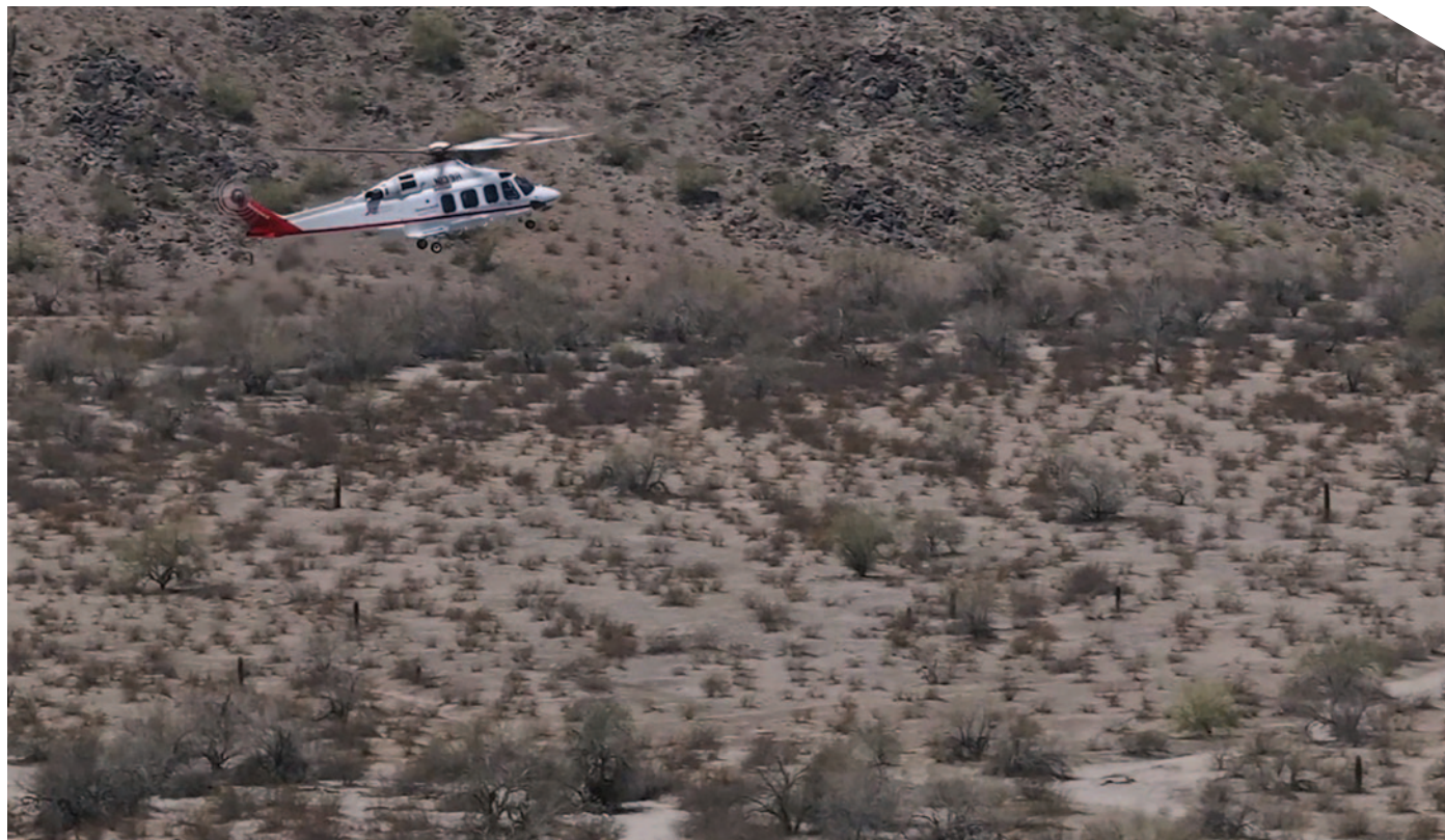
▲ In May 2025, in Phoenix, Arizona, Near Earth Autonomy completed the first autonomous test flight of a Leonardo AW139 helicopter as part of the U.S. Marine Corps's Aerial Logistics Connector (ALC) program. (Image courtesy of Near Earth Autonomy.)
