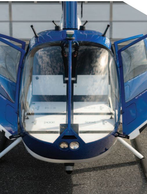
Top to bottom: Rotor Technologies chose the popular Robinson R44 as its primary platform. They sell a retrofit package to convert this helicopter to an autonomous aircraft.
