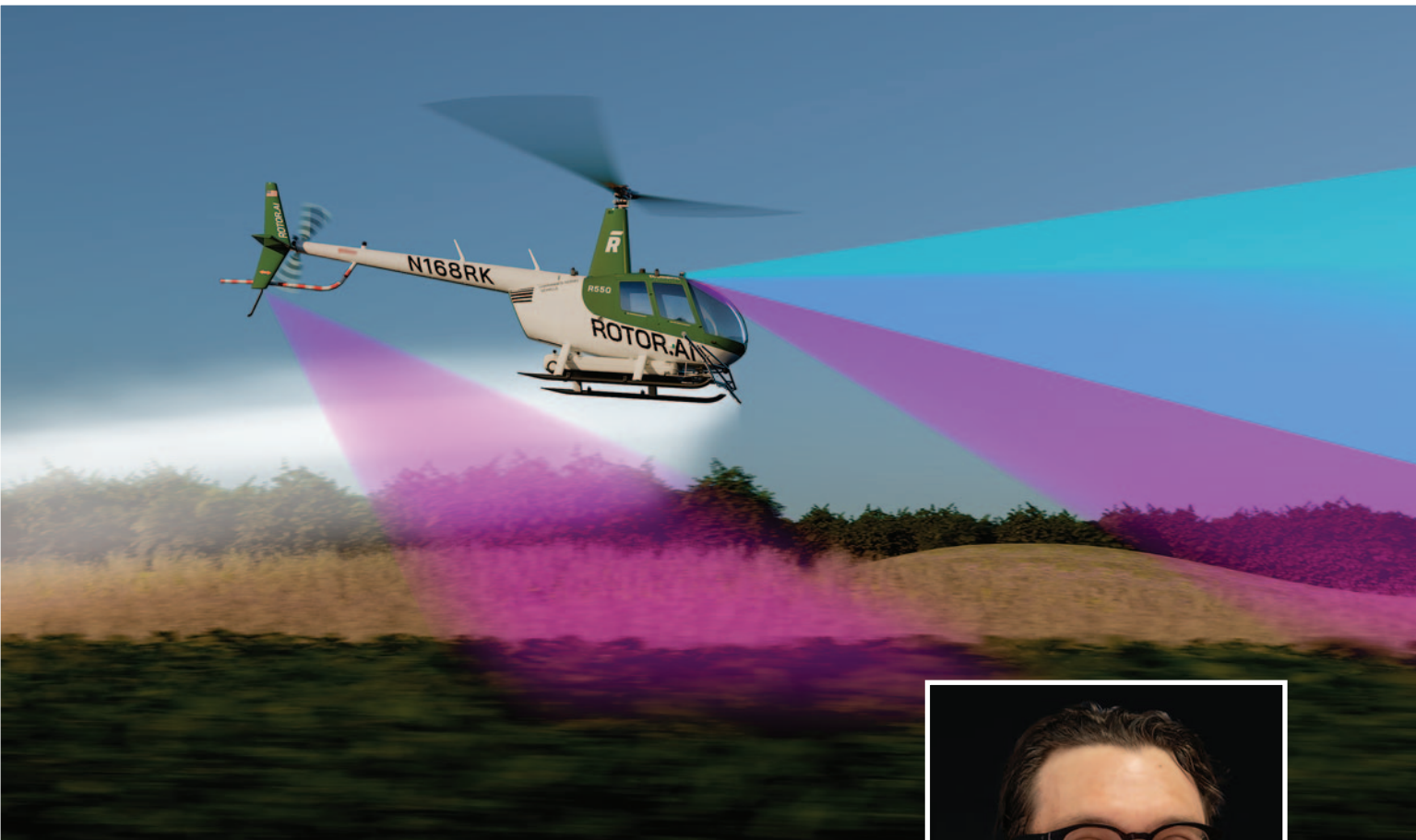
▲ Part of the retrofit process is to add new sensors to the helicopter to give it independent awareness of its surroundings. (Image courtesy of Rotor Technologies.)
