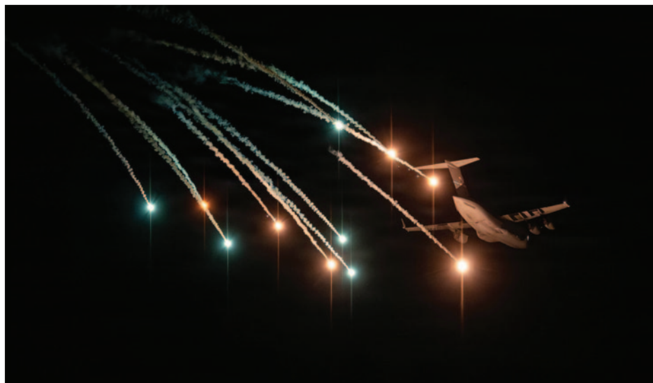
◀ A C-17 Globemaster III conducts flare testing operations at Eglin Air Force Base, Florida, earlier this year. Eglin units coordinated flare-testing operations to evaluate and field improved defensive-system capabilities for U.S. Air Mobility Command aircraft. (U.S. Air Force photo by Master Sergeant J.D. Strong II.)
