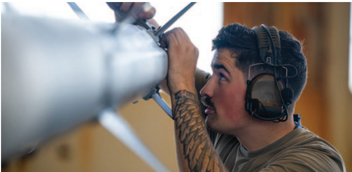
Senior Airman Mathew Morava, a member of the 96th Aircraft Maintenance Squadron, secures fins onto an AIM-120 missile during a weapons load competition. (Photo by Samuel King, Jr., courtesy of the U.S. Air Force.)
