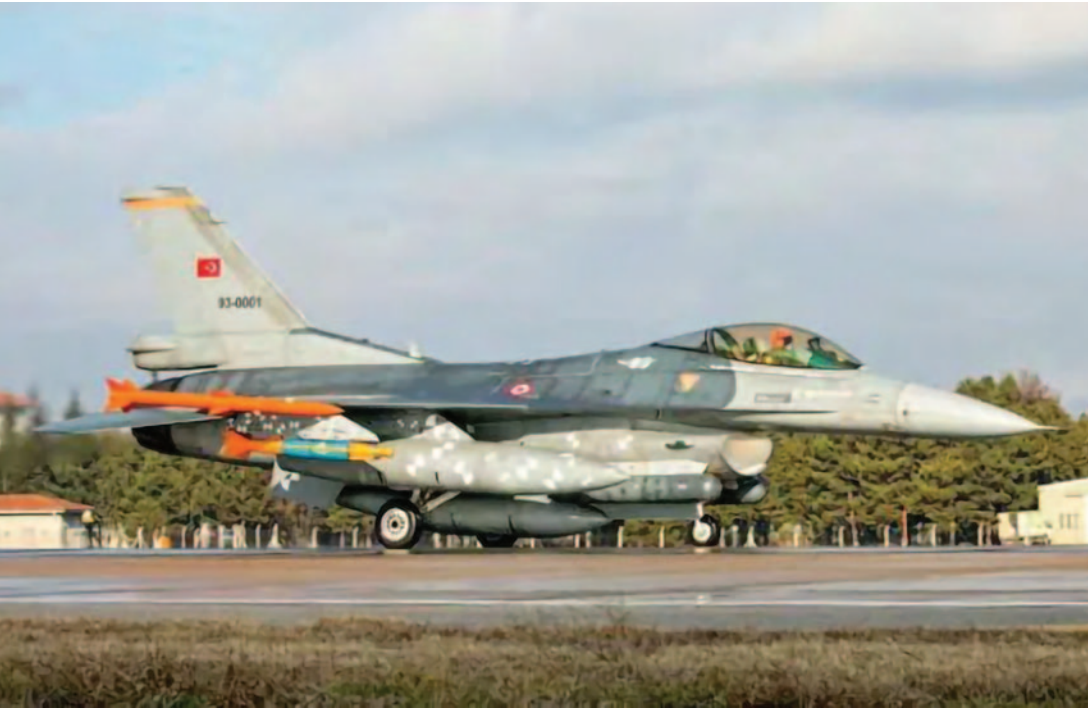
An F-16 Fighting Falcon assigned to the 85th Test and Evaluation Squadron taxis after flying with the Integrated Viper Electronic Warfare Suite (IVEWS) for the first time at Eglin Air Force Base, Florida. (U.S. Air Force photo by 1st Lieutenant Rebecca Abordo.)
