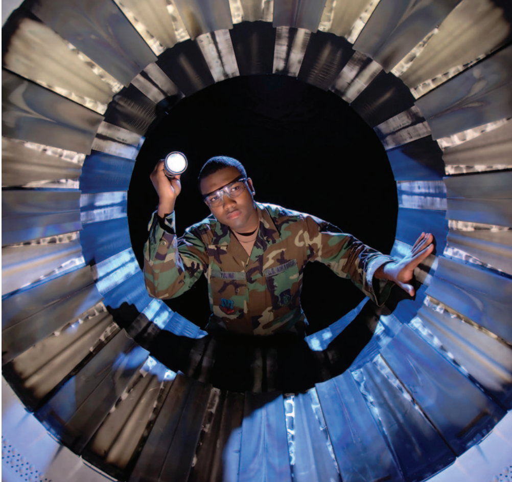
Airman 1st Class Jacques Young of the 158th Fighter Wing inspects the turbine blades (dubbed “turkey feathers”) on an F-16 Fighting Falcon’s Pratt and Whitney F100-220E engine. (U.S. Air Force photo by Master Sergeant Rob Trubia.)
