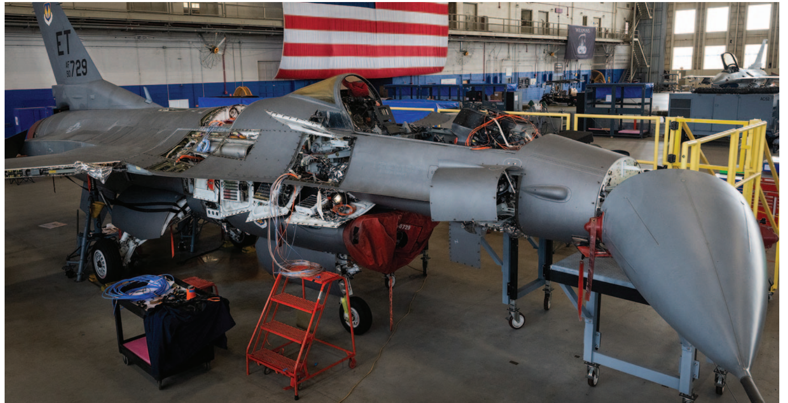
An F-16 Fighting Falcon undergoes modifications as part of the Viper Experimentation and Next-gen Operations Model. The changes include software, hardware, and instrumentation that will enable the aircraft to fly autonomously. (U.S. Air Force photo by Samuel King Jr.)
