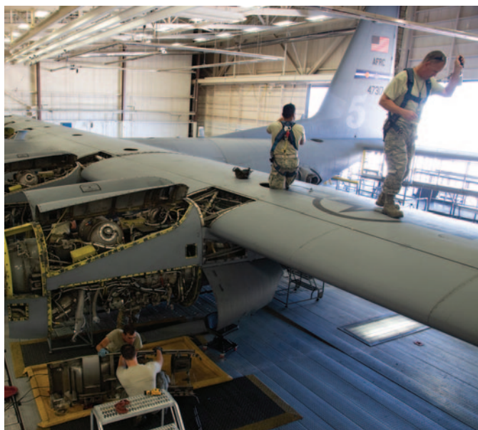
Reserve Citizen Airmen with the 302nd Maintenance Group examine a C-130 Hercules aircraft during an isochronal inspection at Peterson Air Force Base, Colorado, in summer 2019. Maintenance, repair, and overhaul technicians are among the main beneficiaries of the proliferation of predictive maintenance systems. (U.S. Air Force photo by Technical Sergeant Frank Casciotta.)
