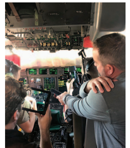
Extended reality (XR) training tools include detailed virtual recreations of real-world environments. Here, Jesse Matos, a Mass Virtual team member, and Thomas Torbert, Air Mobility Command Logistic Management Specialist, scan a flight deck of C-130J Super Hercules to create an environment for training of 19th Air Wing maintainers at Little Rock Air Force Base, Arkansas, in 2019. (Image courtesy of the U.S. Air Force.)
