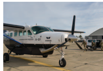
Airmen shown loading weather equipment into Xwing's autonomous Cessna 208B Grand Caravan during AGILE FLAG 24-1, held in January at McClellan Airfield in Sacramento, California. Smaller aircraft like this help ensure autonomous flight technology is developed and tested before being used on larger platforms like the C-130. (U.S. Air Force photo by Matthew Clouse.)
