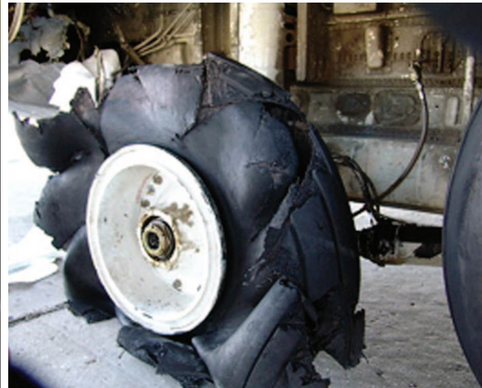
After landing at Contingency Operating Base (COB) Speicher in Iraq, the brakes overheated on this Wyoming Air National Guard C-130. Crew members used water to cool the brakes and prevent a fire. (Image courtesy of the U.S. Air Force.)
