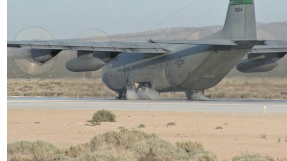
A C-130E from the 19th Airlift Wing at Little Rock Air Force Base, Arkansas, comes to a screeching halt during a Wheel Brake System Improvement test, held in May 2011, at Edwards Air Force Base, California. The C-130 was on loan to the 418th Flight Test Squadron to test new carbon brakes and the Mark IV Digital Antiskid Control Unit. (U.S. Air Force photo by Doug Spinks.)
