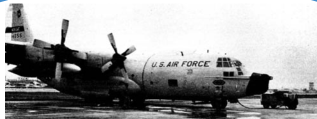
A U.S. Air Force HC-130 outfitted with the AN/ARD-17. (Image courtesy of NASA.)
