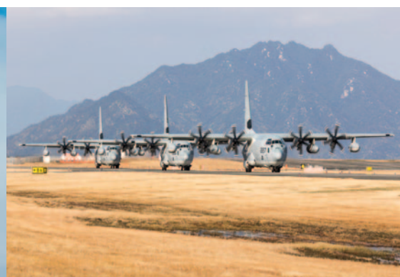
The U.S. Marine Corps uses the KC-130J for in-flight refueling of other aircraft, ranging from helicopters to fighters, as well as for forward refueling of ground vehicles. (U.S. Marine Corps photo by Corporal Jackson Ricker.)
