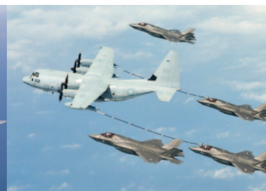
Four F-35s tank off of a Marine Corps' KC-130J. (Photo courtesy of Lockheed Martin.)
