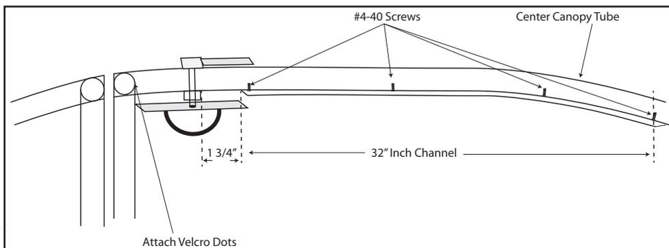
3. Install the wire bows in their respective locations, and bend them by hand to conform to the canopy shape. The ends should just lightly touch the canopy.
