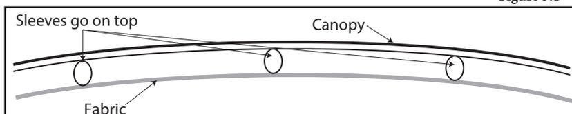
8. After installing the six Velcro dots, stick the Velcro patches on the fabric to the dots, and adjust the front thumb screw so there is just a slight amount of tension on the front fabric panel. Then extend the #5 bow to the rear and lock the thumb screw. Extend the back two panels and lock the back white thumbscrew. The shade is now in its normal extended position. The rear two panels are normally not moved when using the SunShade.
