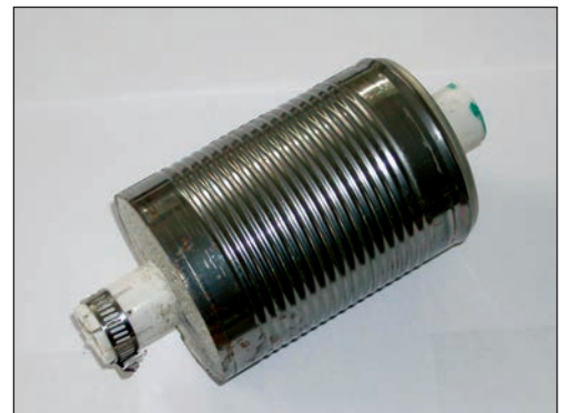
Figure 1: A "soup can" counterweight for the Gizmo made from a split PVC pipe and a stainless steel hose clamp. The can is filled with cement. (Courtesy: VA3KSF/KB1SF)
