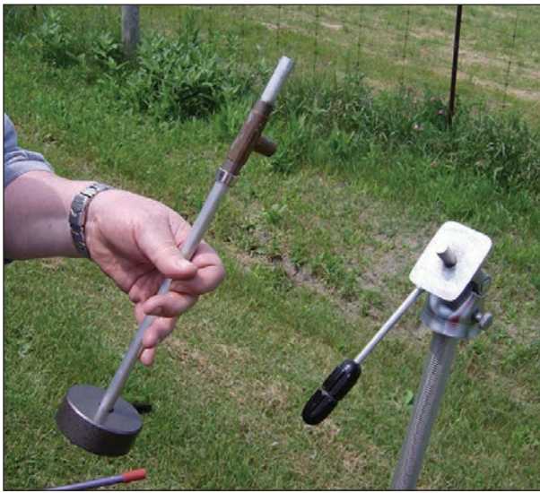
Figure 3: Here's the basic Gizmo with the counterweight, main shaft, copper Tee and bushings installed. Note the drill stop between the Tee and the weight. This addition is not necessary, but Art finds it handy so that the shaft doesn't slide in the Tee when attached to the antenna. Also note the short stub attached to the tripod. (Courtesy: VA3KSF/KB1SF)
