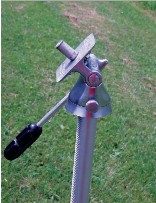
Figure 4: This photo shows the short stub screwed into the tripod head. The angle of maximum elevation of the upcoming satellite pass is set with the tripod's elevation control. Here it's set to about 45 degrees. (Courtesy: VA3KSF/KB1SF)
