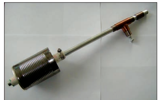
Figure 2: The "soup can" counterweight mounted on the Gizmo. (Courtesy: VA3KSF/KB1SF)
