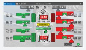
Instant access to critical tasks, with a predictive alignment flow that provides only the steps you need.
