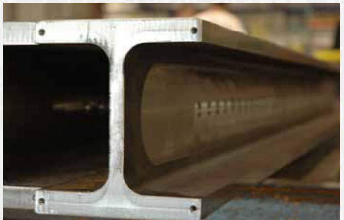
Column Construction, One Piece Beam with Machine Safety Lock Location
