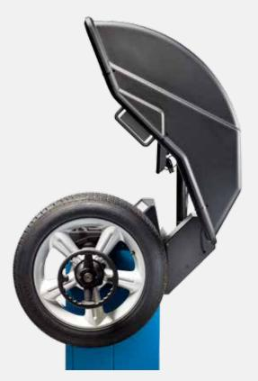
**Space-Saving Wheel Guard** Flat back panel allows for placement directly against a wall, reducing footprint to save space in the shop.
