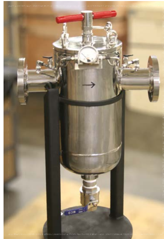
Fabricated Basket Strainer
