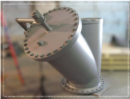
Fabricated "Y" Strainer
