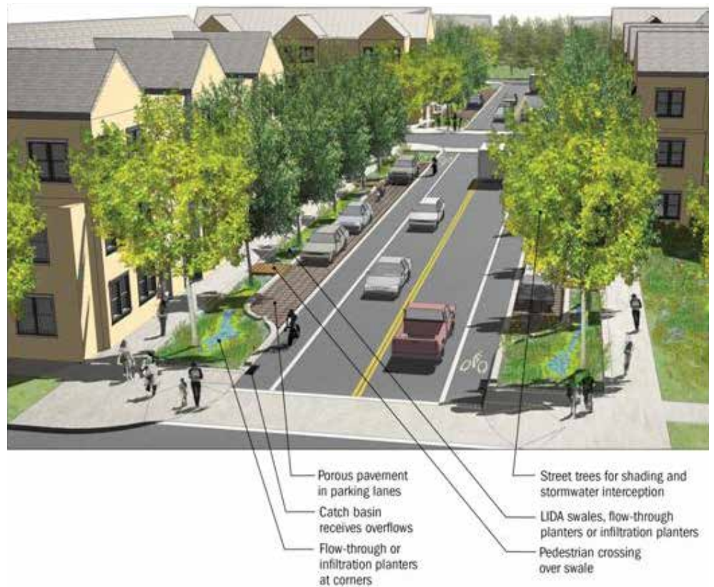
Figure 67. Greener Streetscape using LID practices. Source: “ Greening the Code ” Washington County, OR.
