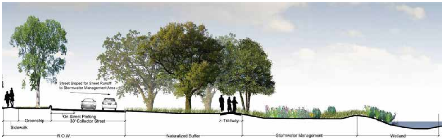
Figure 64. Stormwater Treatment Train within Conservation Development.
