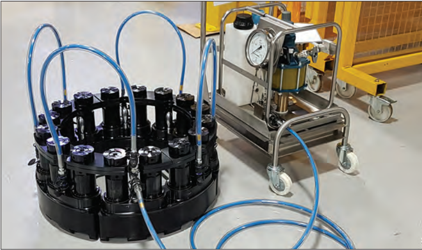
▲ Multi Stud Tensioning Set-Up.
