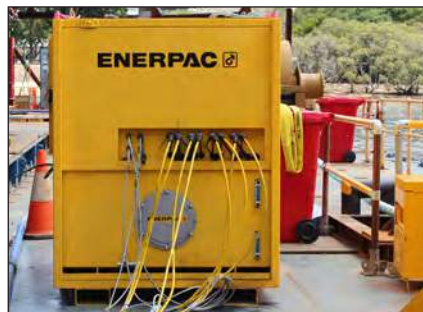
▼ SyncHoist Powerpack to operate the 4 lifting points.
