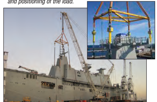
▼ A SyncHoist system used to align steel blocks of the ship's control tower sections allowing gradual lifting and positioning of the load.
