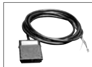
251660 – Foot switch with 3,1 m cord. Single pole, double throw, 15 amp @ 125-250V. Wt., 0,5 kg.
