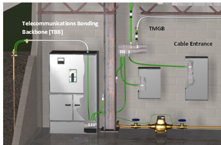
Figure 1 – Service Entrance Grounding
