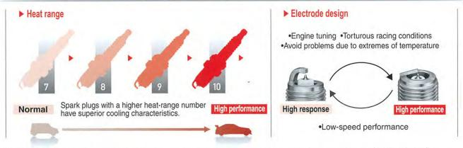
Racing plugs for both two- and four-wheel vehicles have been developed and designed for use in engines that have been finetuned to achieve maximum power under specific racing conditions. Racing plugs differ from standard plugs, both in appearance and performance, and often sacrifice plug life, and efficiency at low-speeds for optimum performance and durability under torturous racing conditions. Racing plugs do not improve output.
