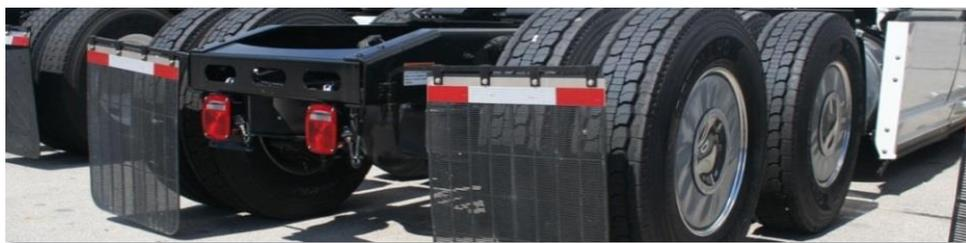
Our custom mud flaps are available in heavy duty rubber and plastic (polyethylene) in a variety of sizes, colors and thicknesses.
