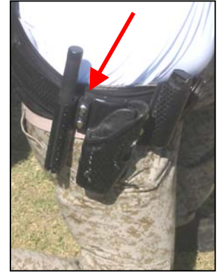
A keeper is placed between the baton and the holster to prevent the baton from interfering with the draw.
