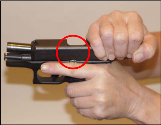
Line right thumb with locking notch on slide
