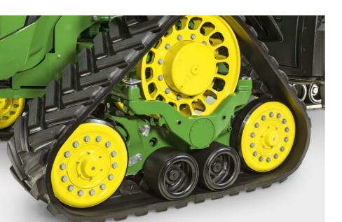
4,57 m² ground contact area are benchmark in this hp class. Even fully ballasted, the static ground pressure at the rear is as little as 36 kPa. Soil berming at the headland is almost not existent, although the turning radius is even smaller than on a 8 Series wheel tractor.
