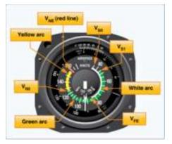
You're at the yoke of your private airplane. There are certain airspeeds that should be very important to you. The recommended speed at which you should take off, a recommended speed at which you should land, the maximum speed you can fly and make use of full deflection of your controls... and others. But how do you know what your airspeed is? You monitor the airspeed indicator, of course. This clever device reacts to characteristics
