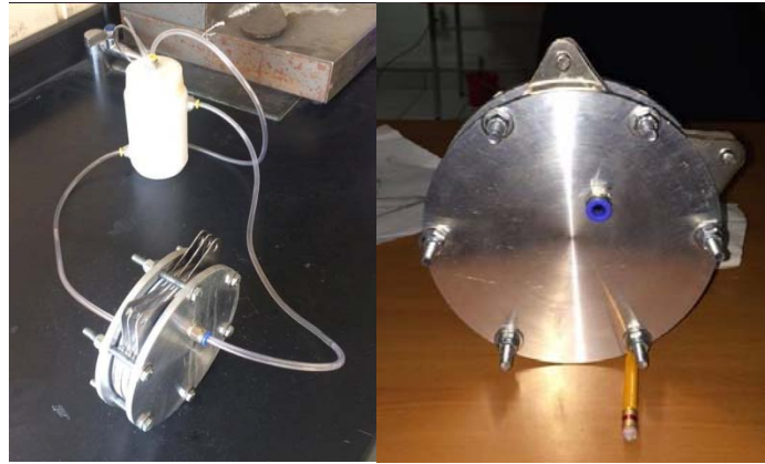
Figure 2- Product – alkaline electrolyzer in performance analysis. Fuente: (Fuentes, 2016)
