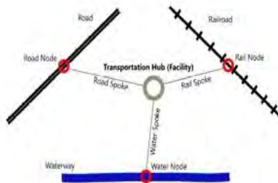
Figure 1: Three transportation networks integrated through intermodal transfer facilities (Swayne et al. , 2010)
