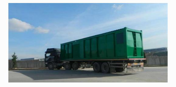
World wide easy and low-cost transport by truck, rail and ship due to international ISO-container- measurements
