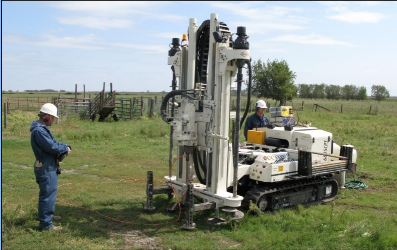
Running HPT logs in the Platte River alluvial aquifer, Clarks, NE.
