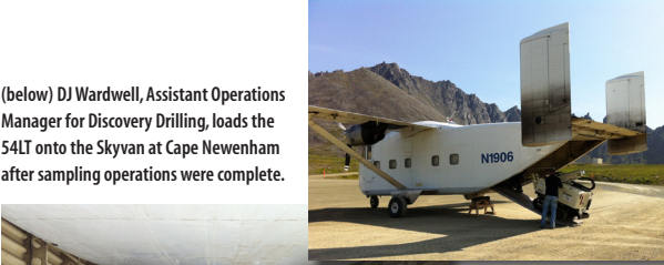
(above) The 54LT’s small size and light weight made it a perfect candidate for remote Alaskan sites with logistical constraints. There was no need to disassemble any part of the rig for transport.
