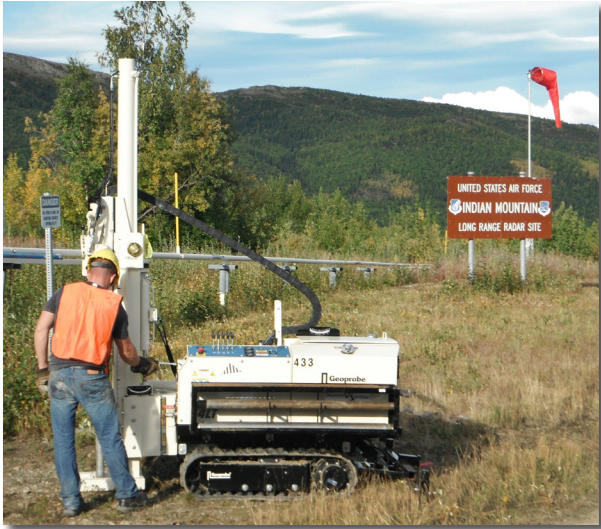
DJ Wardwell with Discovery Drilling uses the 54LT to collect soil samples at Indian Mountain Air Force Station in Alaska near the top of the runway.
