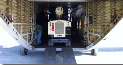
(above) The 54LT’s small size and light weight made it a perfect candidate for remote Alaskan sites with logistical constraints. There was no need to disassemble any part of the rig for transport.
