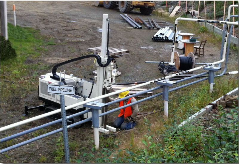
DJ Wardwell uses the 54LT to collect MCS soil samples near an active above-ground fuel line at a site at Indian Mountain in Alaska.
