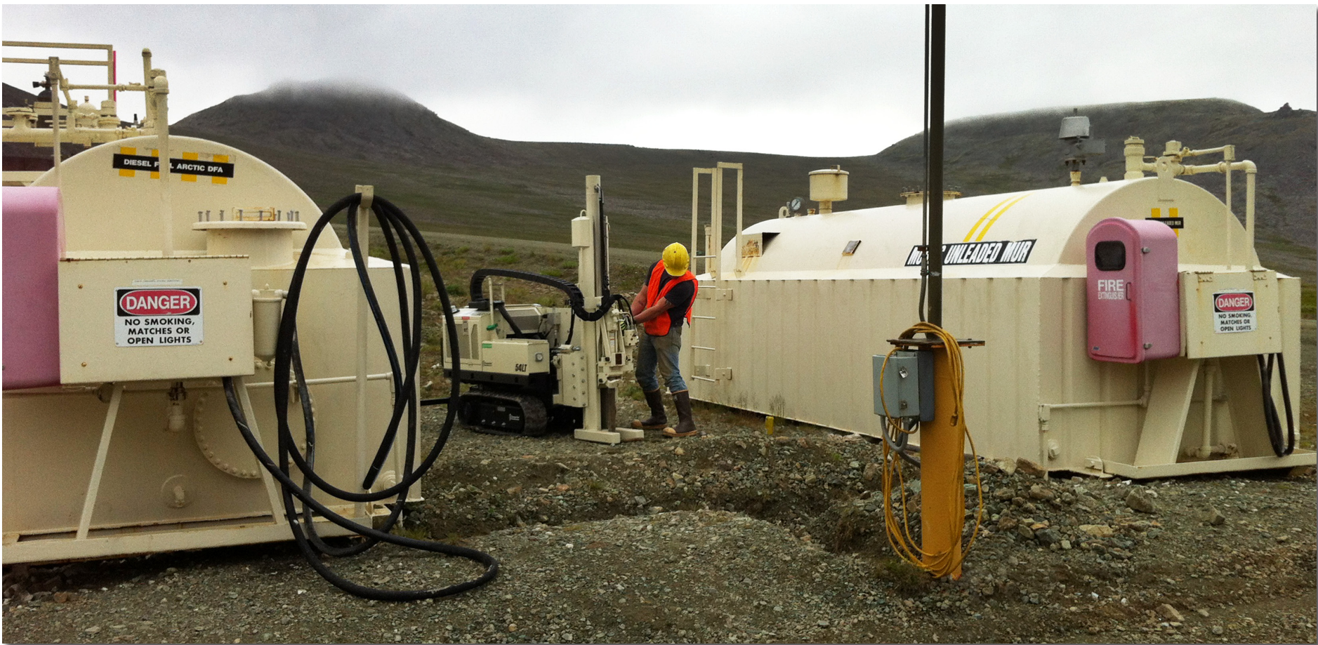
Collecting MCS soil samples between two active fuel storage tanks at Cape Newenham Air Force Station Long Range Radar Site (LRRS) in southwest Alaska.
