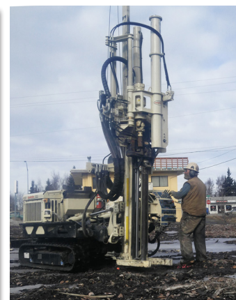
Richard Banzhaf, Driller, collects 3-in. MC7 soil samples using the 7822DT.
