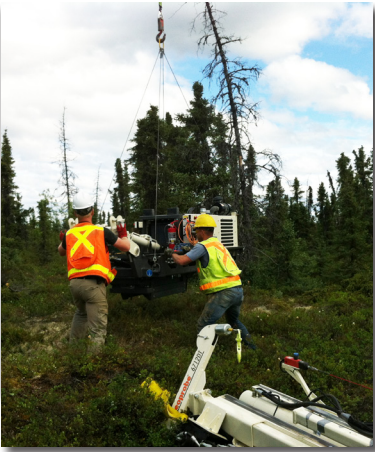
(above right) And finally, using a helicopter long-line system, the power unit of the 6712DT joins the other two sections on the ground.
