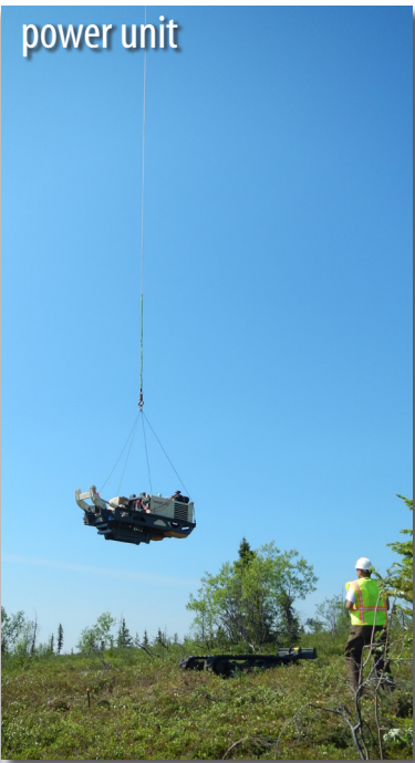
(above right) And finally, using a helicopter long-line system, the power unit of the 6712DT joins the other two sections on the ground.
