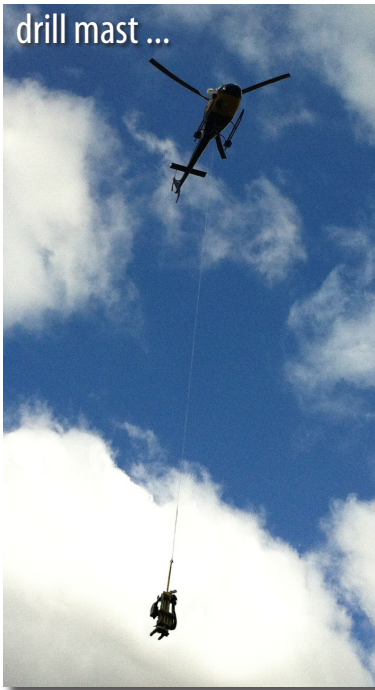
(above left) First the drill mast section of the 6712DT is mobilized to the site via helicopter.
