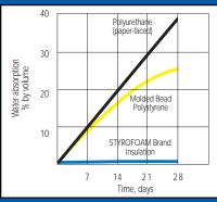
Here, insulating foams underwent temperature and vapor pressure gradients for 28 days. This is one of the most common ways moisture gets absorbed – and again, STYROFOAM brand insulation outperformed the competition.
