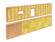
STYROFOAM brand insulation covers the whole wall surface, not just the area between the studs. It provides important insulation over the wood framing, which can account for up to 25 percent of the wall area, and 15 to 42 percent of your home's wall heat loss/gain, depending upon the amount of existing insulation in your walls.
