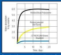
Foam insulations were submerged in water for 21 days while being measured for moisture content. Results show STYROFOAM brand insulation had much less moisture content than other foam insulations.
