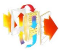
Without STYROFOAM brand insulation on the exterior side of the wall, convective looping occurs in the stud wall cavity, creating heat loss.
