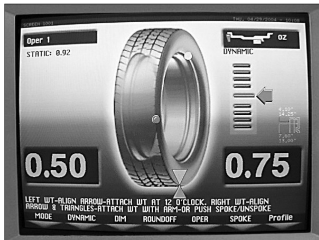
Figure 14 - Weight Placement Arrows in 3D Mode.
