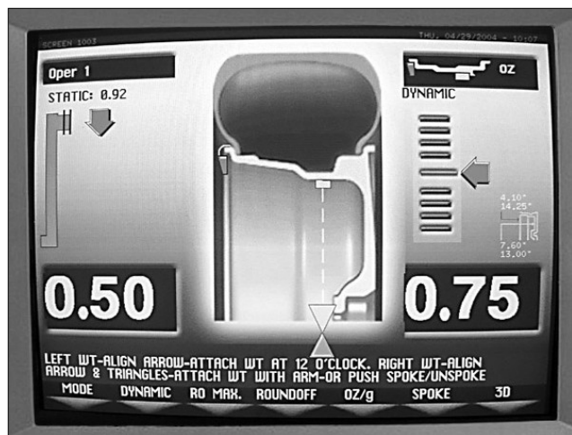
Figure 15 - Weight Placement Arrows in Profile Mode.
