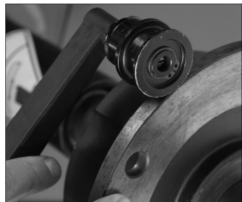
Figure 40 - Offset Arm Gauge to Faceplate
