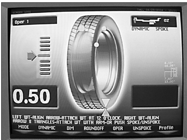
Figure 28 - Spoke Weight Placement Screen
