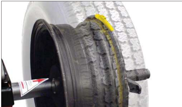
Figure 24 - Calibration Weight On Outboard Flange At Top-Dead-Center
