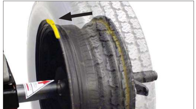
Figure 25 - Calibration Weight On Inboard Flange At Top-Dead-Center
