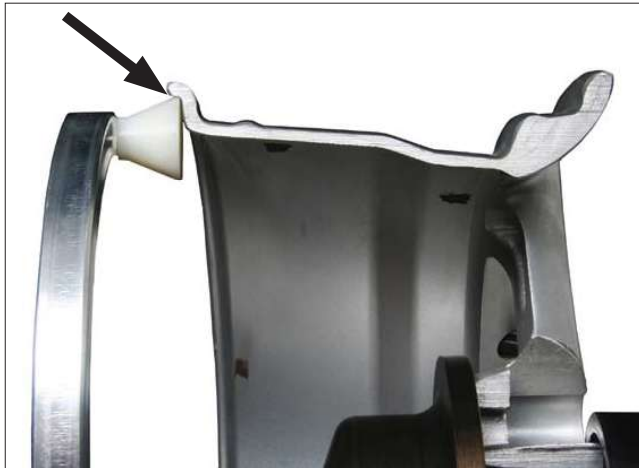
Figure 8 - Clip-on Weight Location Viewed on a Cut-Away Rim for Clarification
