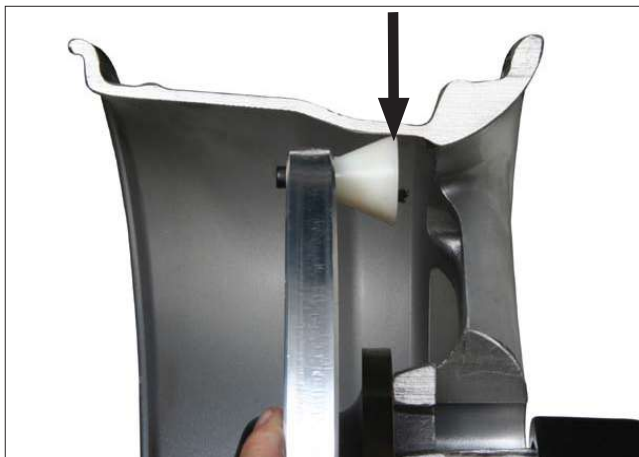
Figure 9 - Hidden Weight Location Viewed on a Cut-Away Rim for Clarification
