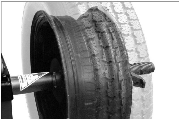
Figure 20 - Calibration Weight On Outside Flange At Top-Dead-Center
