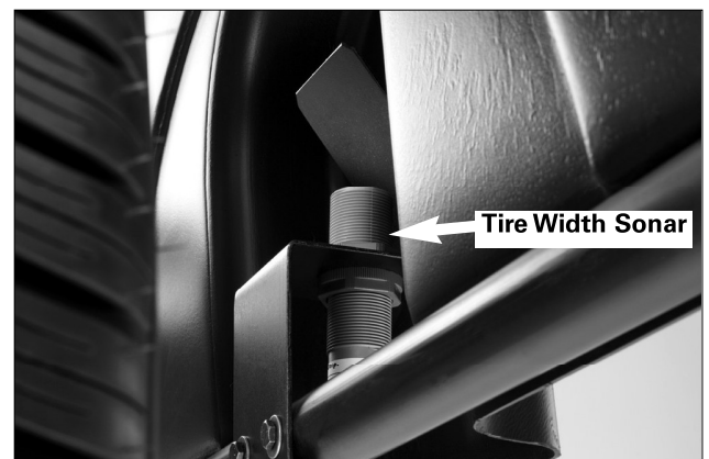
Figure 10 - Tire Width Sonar Located Inside Hood
