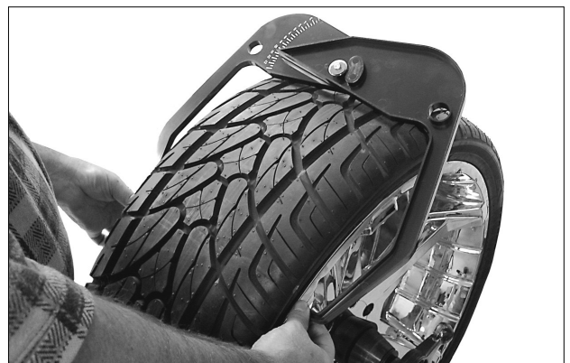
Figure 13 - Caliper Placement On Wheel
