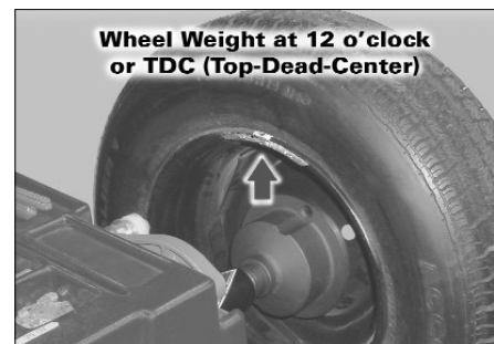
Figure 46B - Test Weight Inside Flange Position
