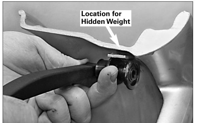
Figure 9 - Hidden Weight Placement Location Viewed on a Cut-Away Rim for Clarification.
