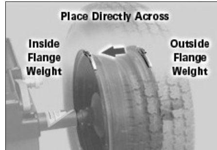
Figure 46A - Test Weight Inside Flange Position
