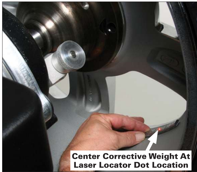
Figure 11 - Centering Corrective Hidden Weight At Laser Locator Dot Location
