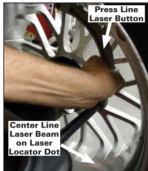
Figure 9 - Positioning Line Laser Beam At T2 - Tape Hidden Weight Location (A2)
