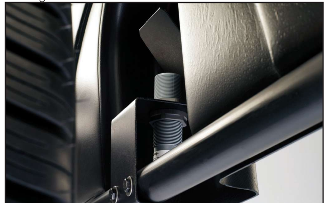
Figure 10 - Tire Width Sonar Located Inside Hood
