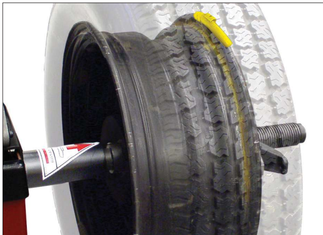
Figure 20 - Calibration Weight On Outside Flange At Top-Dead-Center
