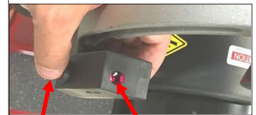
Figure 17 - Centering Corrective Hidden Weight at Laser Dot Location.
