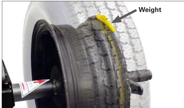
Figure 40 - Calibration Weight On Outside Flange At Top-Dead-Center
