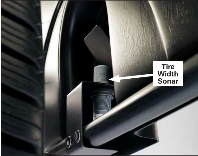
Figure 18 - Tire Width Sonar Located Inside Hood
