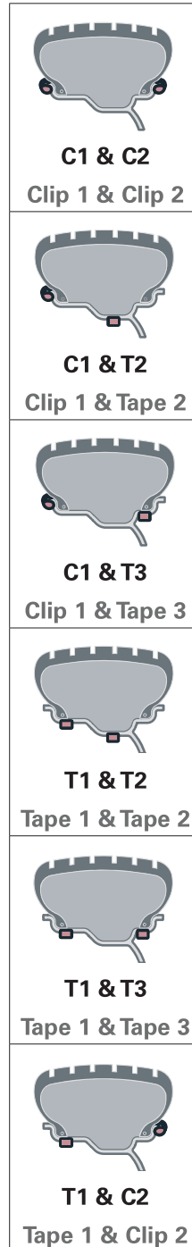
Figure 32 - Dynamic Balance Weight Locations
