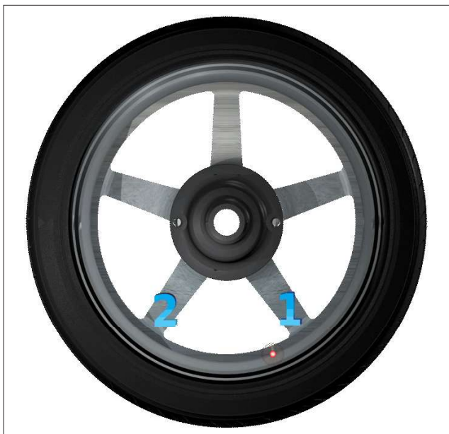
Figure 35 - Spoke 1 and Spoke 2 Locations On Either Side Of Original Outboard Weight Location
