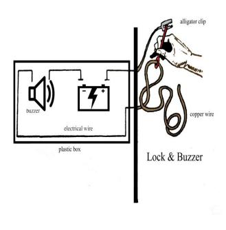
To represent IFGS lockpicking, a lock and a buzzer are connected to form an open, complete circuit (see diagram), which will only close if a character touches their lock pick to the bare copper wire of the lock. The buzzer apparatus is usually contained in a portable box that can be moved from encounter to encounter if needed.
