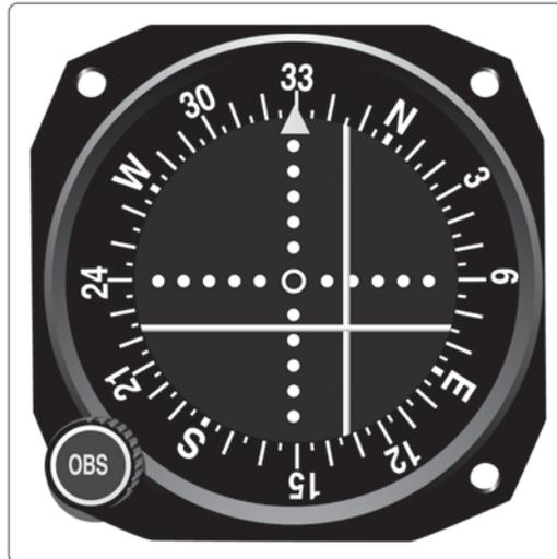
Figure 141. – OBS, ILS, and GS Displacement.
