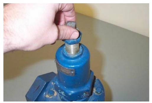
Remove the spring chamber #6, top spring washer #4, springs #5, and bottom spring washer #9.
