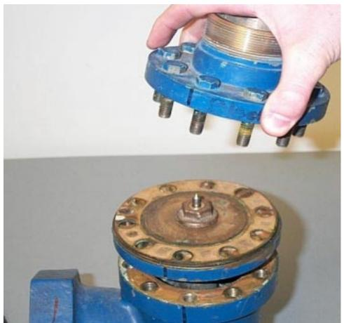
Remove the pilot assembly (including the diaphragm nut #10, diaphragms #11, pilot pin #12, pilot valve #13, and o-ring #25) and re-pack as follows:
