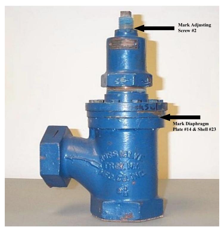
Loosen the adjusting screw #2 in order to release the compression on springs #5. (Note: There is no need to remove the adjusting screw completely.)
