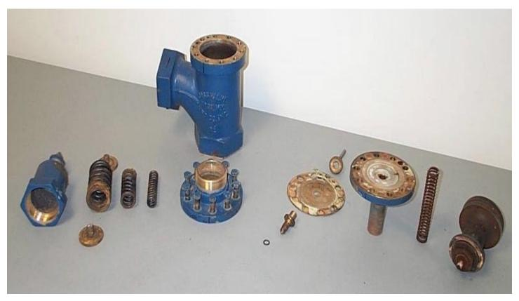
Re-install the stem assembly and guide spring #17.
