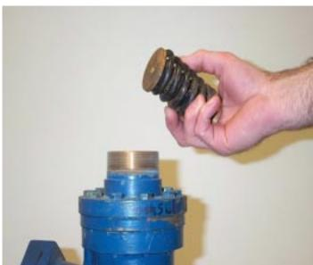
Loosen the assembly bolts #30 and remove the diaphragm cover #8.
