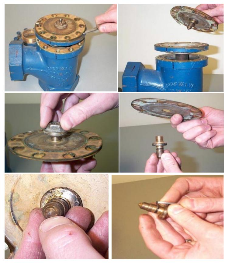
Remove the diaphragm plate #14 and inspect as follows:
