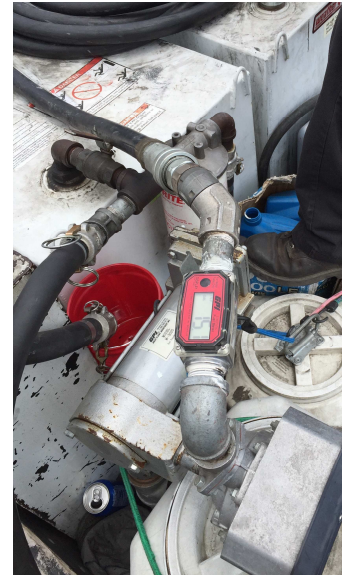
External fuel drain fitting.
