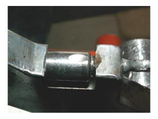
TEST VII: With 10 percent of BestLine mixed with PENNZOIL 5W-30. Using BestLine's additive, at only 10%, with a 5-pound weight, there was no visible wear scar. It took thirty (30) seconds on the bench test to create a measurable loss, which was then only .02 grains (or .006 grains for 10 seconds).
