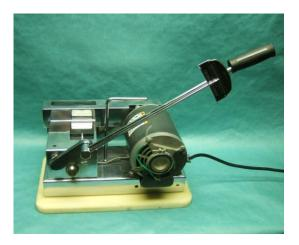
Using only a five (5) pound weight on the torque wrench, all tested oils and additives (except BestLine's) resulted in failure and significant damage to the "test bearing" in as little as ten (10) seconds. A visual review of the test bearing makes this abundantly clear.
