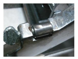
TEST II: With CASTROL GTX START UP 5W-30. Again, the wear scar shown was from only 10 seconds of running with the pressure of a 5-pound weight
