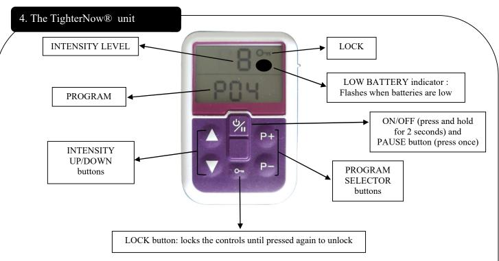
auto-off function: the unit will shut off automatically if, while the unit is turned on, the intensity level is at zero for more than five minutes.
