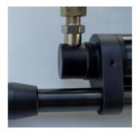
Attach the stainless steel fill adapter to the correct fill euipment. Rotate the fill port's protective cover to allow access. Insert the fill adapter into the fill port.
