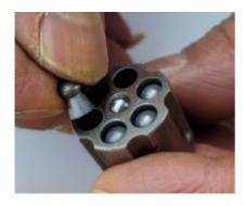
Front of mag shown. Insert a rear of pellet into magazine
