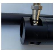
When charging is complete, bleed the excess air using the fill apparatus bleed screw and remove the fill adapter from the rifle.
