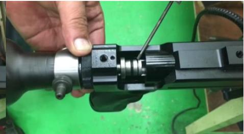
**Put & turn cylinder in and keep 0.5mm~ 1mm gap between barrel and valve.**
