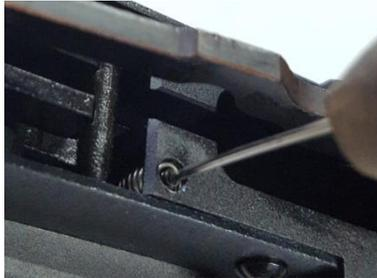
**Using a 0.89 mm Allen key, turn the screw clockwise to decrease trigger pull weight and counter-clockwise to increase trigger pull weight.**
