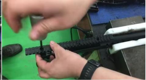
**Take out mounts with releasing two screw**
