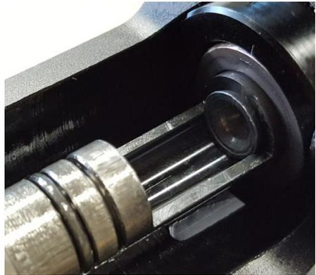
**Insert pellet and push pellets to breeze of barrel & properly seat pellet. If the pellets skirt is not flush with the barrel the accuracy will be poor.**
