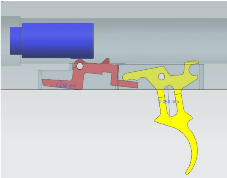
**\*\*\* Do not over-adjust, as this may cause the gun to fire prematurely, not operate correctly and make the rifle unsafe. \*\*\***
