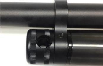
**Attach the stainless steel fill adapter to the correct fill equipment. Rotate the fill port's protective cover to allow access. Insert the fill adapter into the fill port.**
