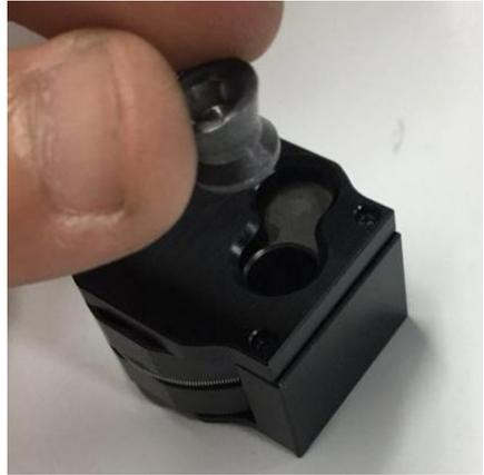
**Insert a pellet into the hole on the lower left**
