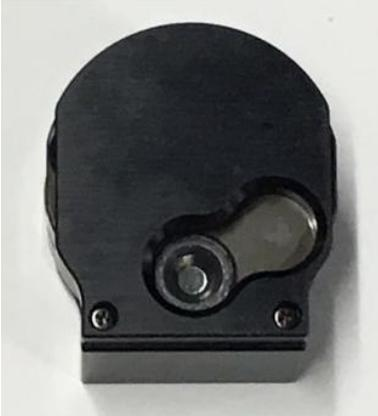
**First pellets has been inserted & properly seated**
