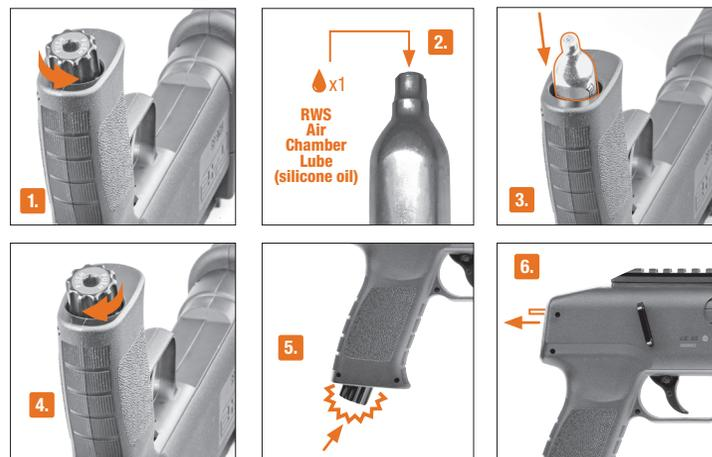
If the marker does not make a popping noise after pulling the trigger, the CO<sub>2</sub> is not being discharged. If indicator pin is not extended (see Section 4, Step 5), check that piercing screw is tight and make sure to strike it to pierce the capsule.
