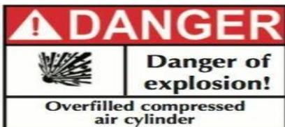
Do NOT exceed maximum fill pressure of 250 bar at room temperature!
