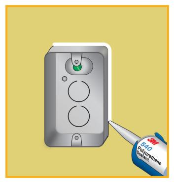
**1.** Apply 3M<sup>™</sup> Polyurethane Sealant 540, 3M<sup>™</sup> Polyurethane Construction Sealant 525 or other compatible sealant around junction box.
