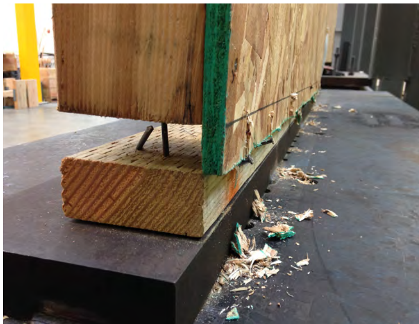
Fastener tearing through sheathing
