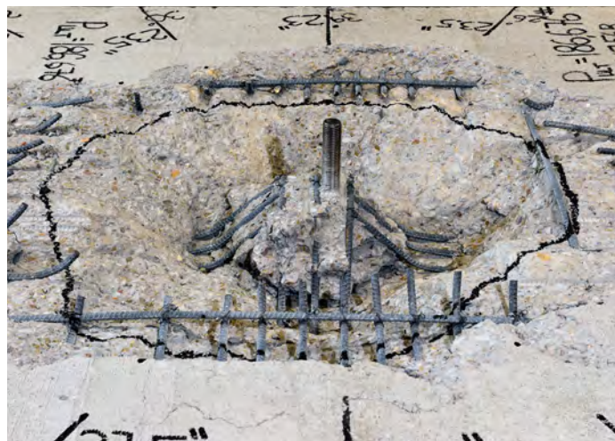
Anchor reinforcement testing at Tye Gilb Laboratory for edge and away-from-edge conditions.
