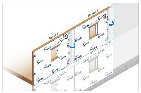
Method 2 – **Tyvek**° **WRB** cut to accommodate additional space between panels based on job site building design
