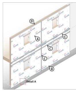
Method 2 – **Tyvek**® **WRB** cut to accommodate additional space between panels based on job site building design
