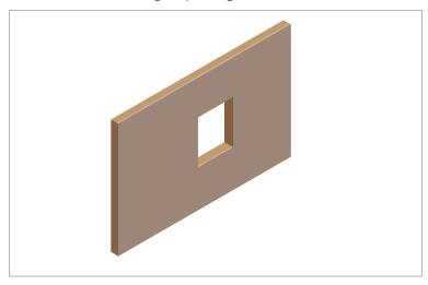
3. Panel with **Tyvek**° **WRB** installed and prepared for window installation
