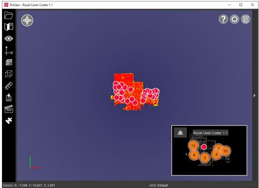
7. Hover over any point to see the coordinates in the bottom left of the window. Note that coordinates can only be shown for points captured by the scanner.
