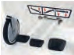
Height and tilt are easily adjusted with handy foot pedals.
